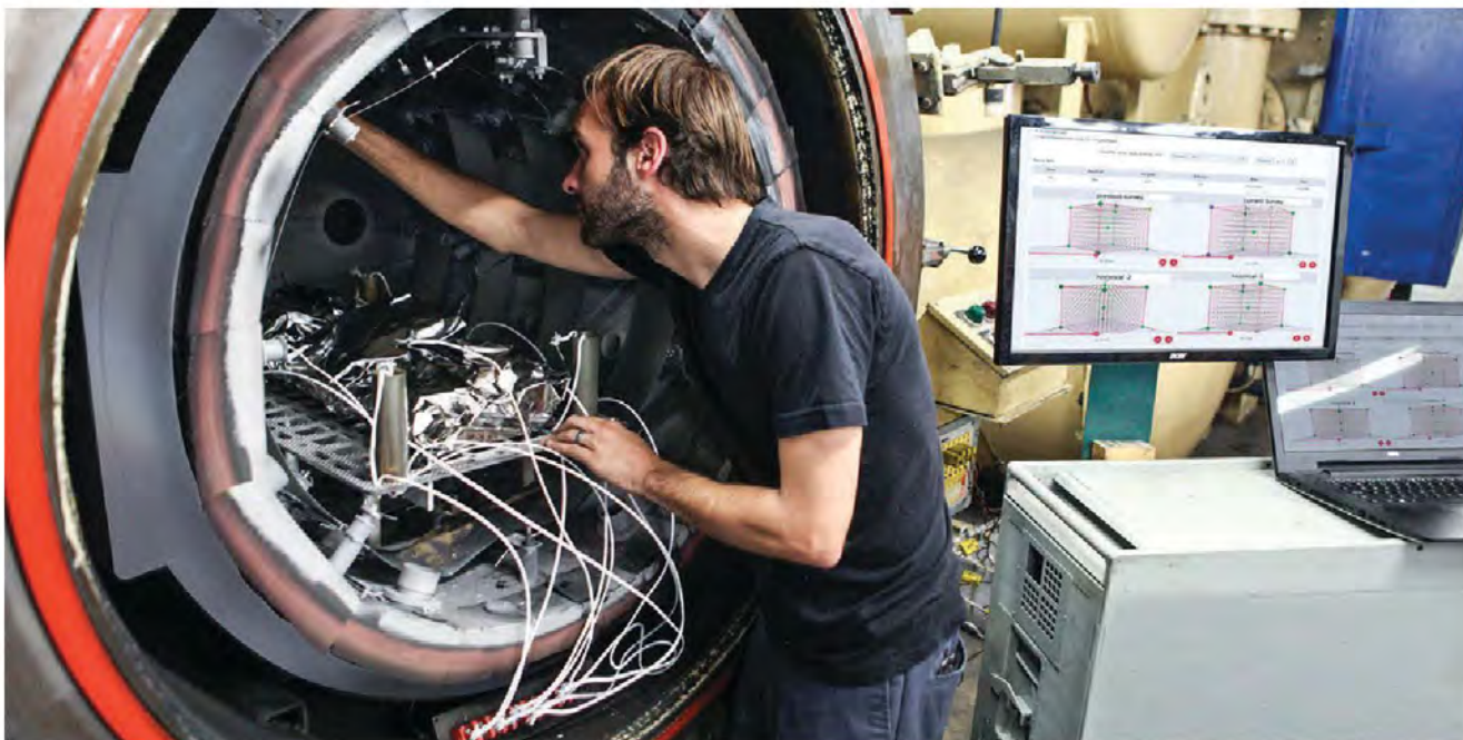
Fig. 4. Eric Reamer shown with vacuum furnace TUS and four-survey display
